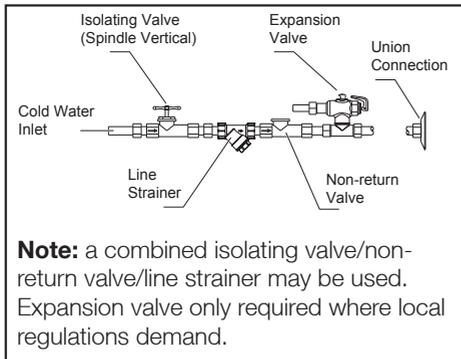
**Note:** a combined isolating valve/non-return valve/line strainer may be used. Expansion valve only required where local regulations demand.
