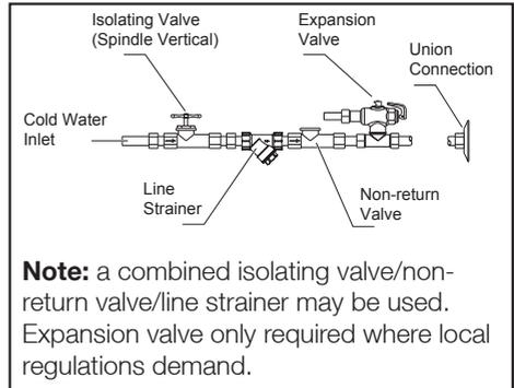
**Note for S.A. and W.A.:** It is a state requirement that a pressure relief valve be fitted on the cold water supply line between the non return valve and the water heater.
