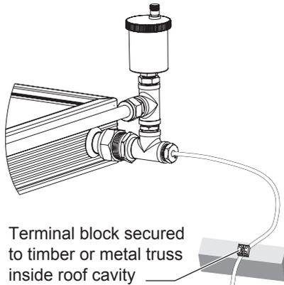
Attach collector sensor cable to terminal block
