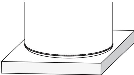
A properly drained overflow tray must be used where property damage could occur from water spillage. (See AS/NZS3500.4 for further details.)
