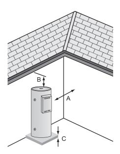
A = 500mm B=300mm C=50mm min For further details, refer to AS5601 – Gas Installation Code
