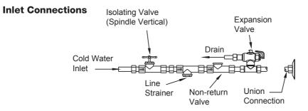
**Note:** a combined isolating valve/non-return valve/line strainer may be used. Expansion valve only required where local regulations demand.
