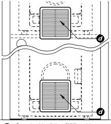
For enclosed installations **ONLY**, a minimum 250 cm<sup>2</sup> of Free Air Ventilation is required.
