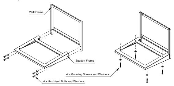
Some minor assembly is required before the wall mounting bracket can be fixed to the wall.
