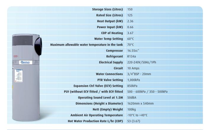
Rated at 20°C, 60% relative humidity ambient and water heated from 20°C to 60°C
