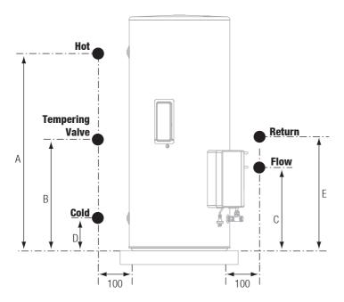
Approximate location of pipework. A tolerance of 25mm is acceptable to dimensions shown in table below.
