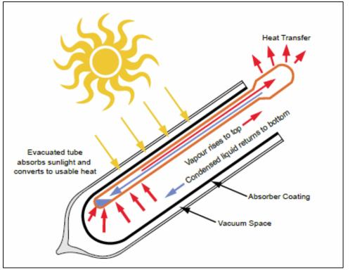
Figure 2 Evacuated Tube Function
