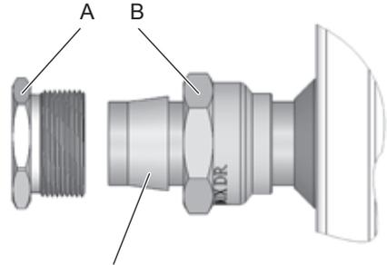
Ensure the brass conetite compression fitting is installed in the correct direction
