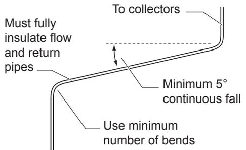
Ensure flow and return pipes from the solar collectors to the water storage tank have a minimum of 5° continuous fall
