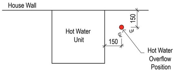
● Approximate location of pipework. A tolerance of 25mm is acceptable to dimensions shown in table below.
