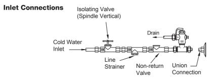
**Note:** a combined isolating valve/non-return valve/line strainer may be used. Expansion valve only required where local regulations demand.
