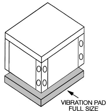
If the unit is installed on a floor over a crawl space, it should not rest on long, unsupported floor joists. Vibrations may be created in the joists with the crawl space acting as an amplifier box resulting in undesirable noise. A drain pan is recommended where water released during start-up or maintenance could cause damage below the unit.
