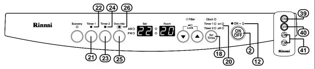
The heater must be between the finishing and starting times of a timer program for the Override to function to work. Either of the Timer indicators (22) or (24) will be illuminated and the Combustion indicator (12) is illuminated green when this is the case. If the Overrrided button (25) is pressed the Override indicator (26) will flash to show that the heater is now operating in override mode. The heater will now start and full manual control will now be available.
