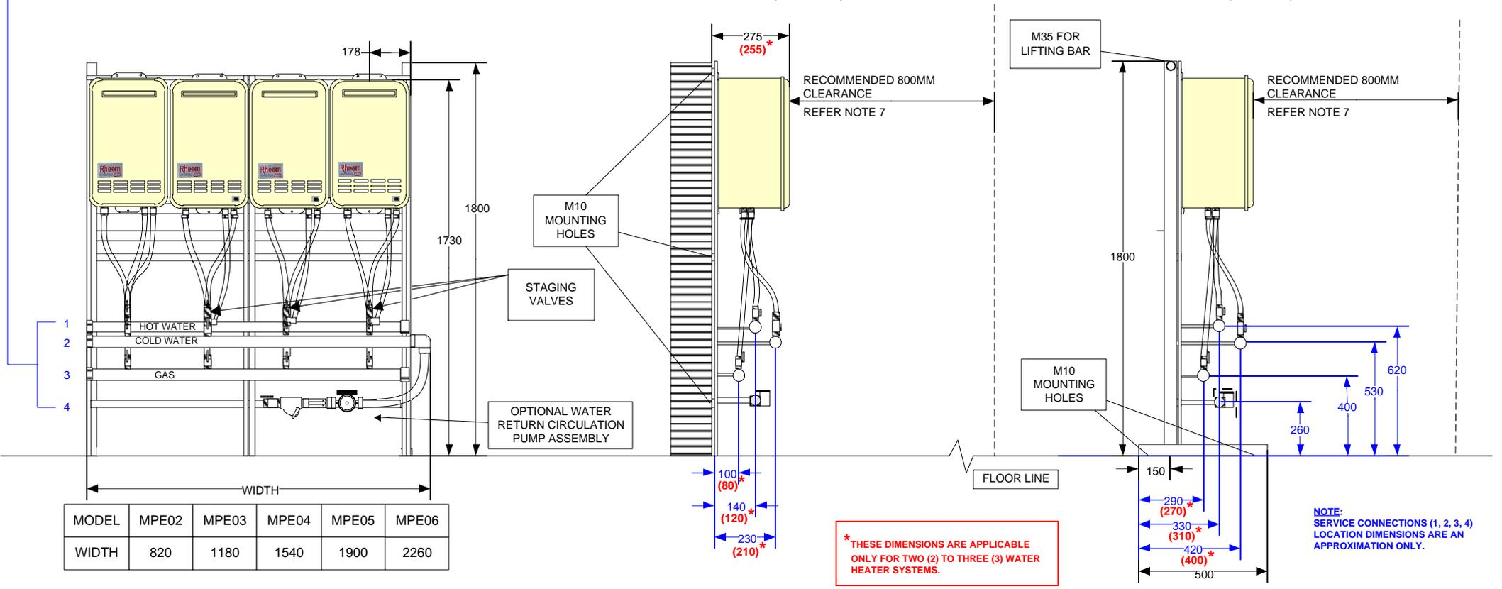
**\* THESE DIMENSIONS ARE APPLICABLE ONLY FOR TWO (2) TO THREE (3) WATER HEATER SYSTEMS.**
