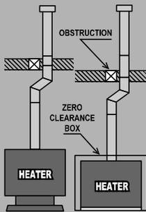
When an obstruction prevents the use of a direct rigid flue run from the appliance to the termination point a FLBEND kit consisting of two 45° offsets can be used to divert the flue.
