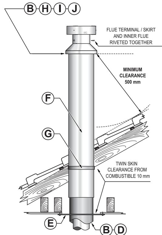
**Flue Terminal Assembly Details**
